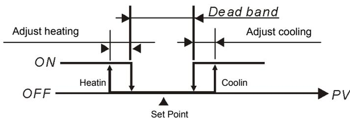
Output of **DEAD** when in PID control mode (Ctrl = PID):
