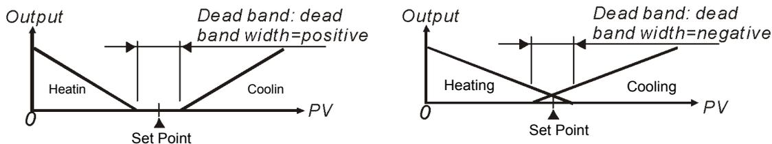
When the controller is in PID control and dual loop output mode, parameter **LoEF** sets the P value of the 2nd set of PID. The 1st set of PID is generated when TUNE = AT, but user can also manually set the PID value. The P value of the 2nd set of PID = the P value of 1st set of PID x **LoEF**. The I and D value of the 2nd set of PID remains the same as the 1st set of PID.
